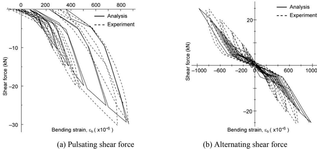
Fig. 4: Shear force-bending strain relations at mid height
