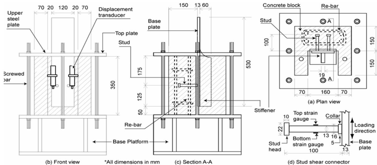
Fig. 1: Specimen details
