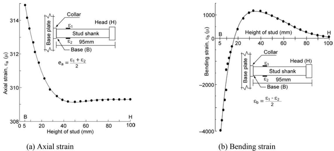
Fig. 5: Strain behavior along mid height of the stud shank
